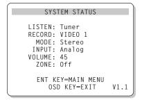
The SYSTEM STATUS menu provides a snapshot of the current system settings and a starting point for reaching all other screens and menus. This screen appears when you press the MENU button on the remote control and displays the following information: LISTEN: the source selected for listening.
